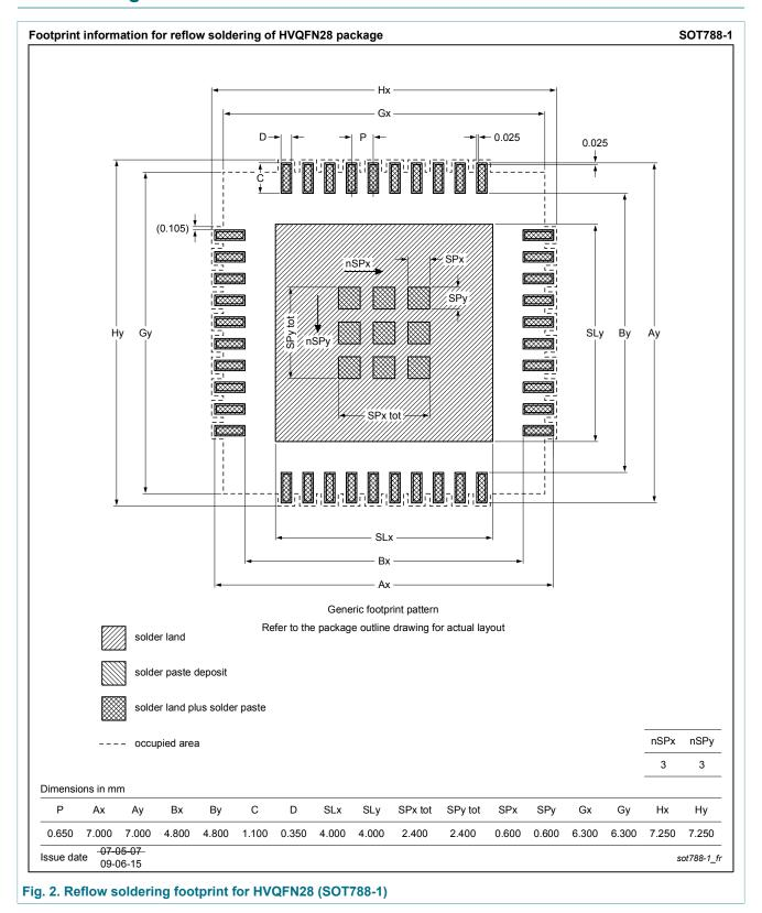
plastic thermal enhanced very thin quad flat package; no leads; 28 terminals; body 6 x 6 x 0.85 mm
