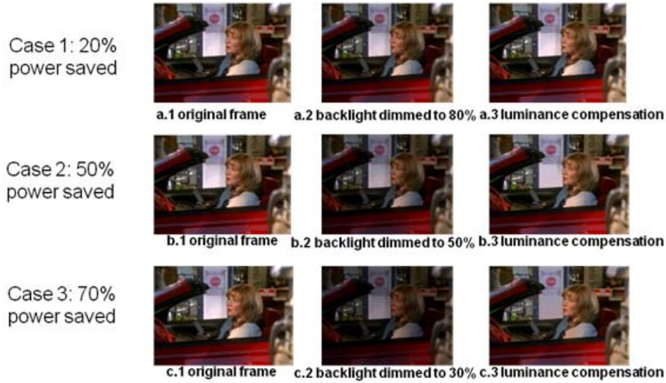
Figure 7. Image Processed with Luminance Compensation and Backlight Dimming
