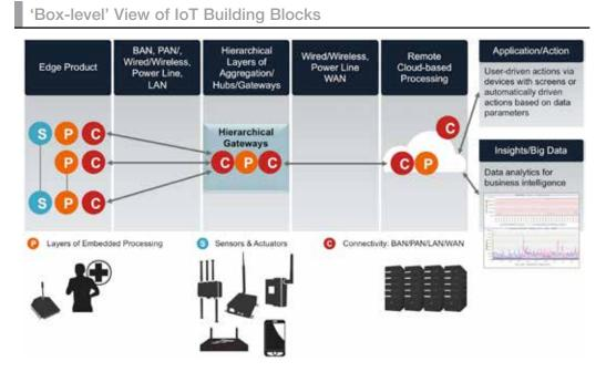
These gateways, in turn, communicate to the cloud via WAN communication technology. Once connected to the cloud through an access network, data will be routed through a server for application/action, as well as big data analysis.
