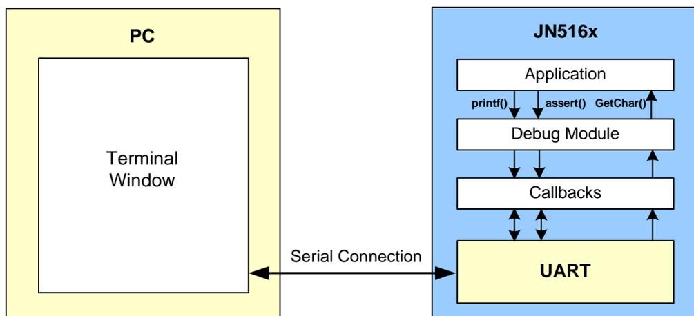
**Figure 9: Typical Hardware Set-Up for Debugging**
