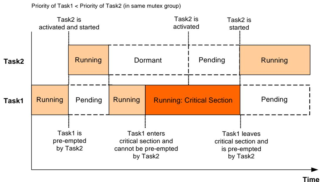
**Figure 3: Mutex Handling of Critical Section**
