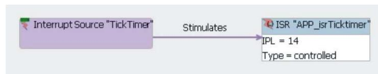
**Figure 1: Linking an Interrupt Source to an ISR**
