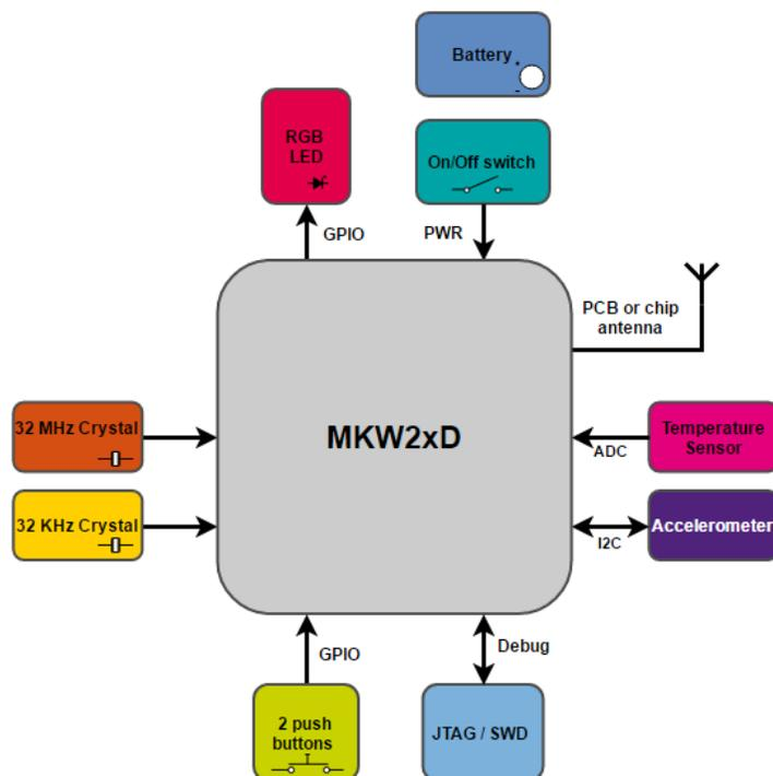
Figure 3. IoT Low Power Sensor Node block diagram
