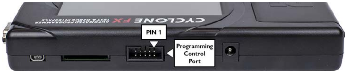
Figure 3-5: Port and Pin 1 Location (Shown on Cyclone FX)
