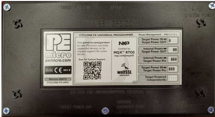
Figure 17-4: Rear Cyclone Case, Five Screws
