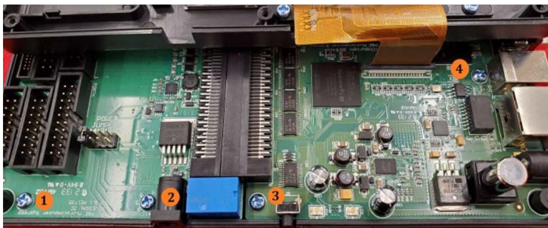
Figure 17-5: Bottom Half of PCB, Four Screws
