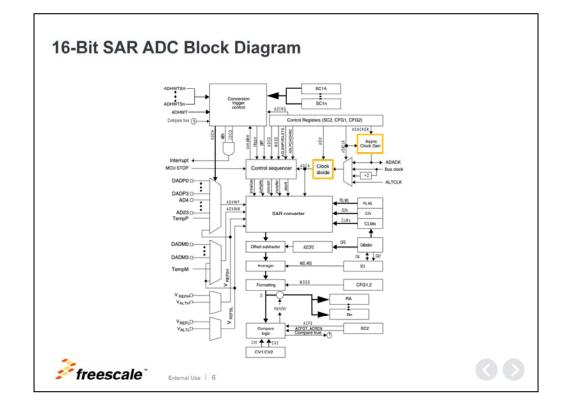
The clock multiplexer and divider generates the ADC source clock, or ADCK. This clock is the reference for the control sequencer and the SAR converter.
