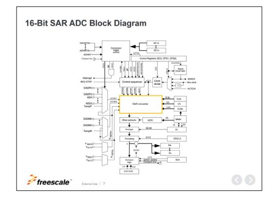
The SAR converter is the heart of the ADC. In this block diagram, the ADC analog input is converted into a digital value.
