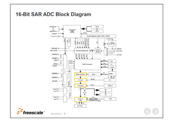
After the SAR converter provides a result, the digital value passes through an offset subtractor, averager, formatting and compare logic; the ADC conversion complete flag, or COCO, is now set.
