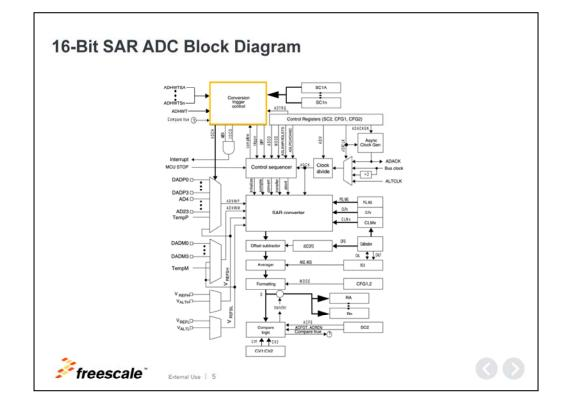
The conversion trigger control handles starting ADC conversion either through software or hardware trigger.
