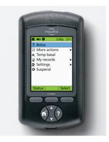
PDM with built-in glucose monitor featuring Freescale's i.MX21 multimedia applications processor and an S08QE8 8-bit MCU.
