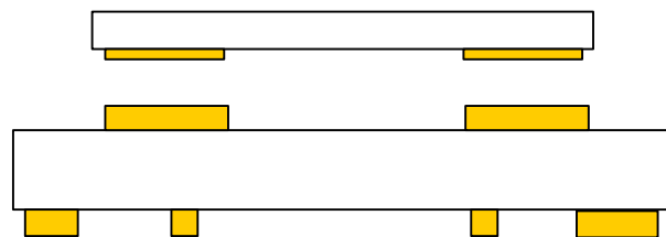
Figure 4. Correct PCB Top Metal Pattern Under Package
