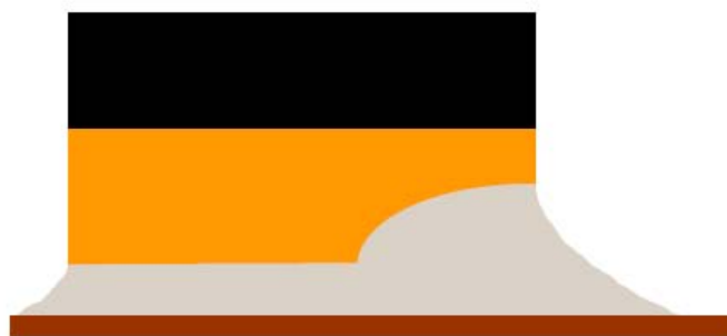
Cross-section of Expected Solder Joint at Half-etch Feature
