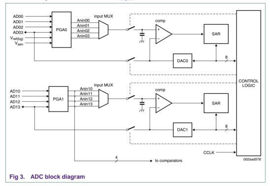
Two 8-bit ADCs are integrated. The conversion speed of the ADC has been improved to 8-bit conversion time of  $\geq$ 1.61 µs at an A/D clock of 8.0 MHz.
